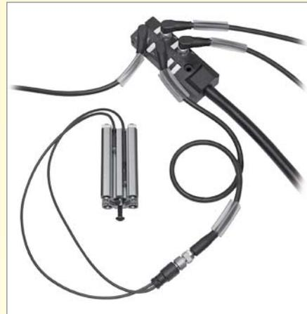
By incorporating passive technology, these blocks concentrate signals into one homerun cordset. The dual density connectors allow for two signals per port. A typical application would include a Balluff V-Twin™ magnetic field sensor used with pneumatic cylinders. The V-Twin provides two sensors with a single connector, which sends both signals through the single cordset back to the high density MIB. This solution reduces sensor and cabling costs without sacrificing reliability or quality.
