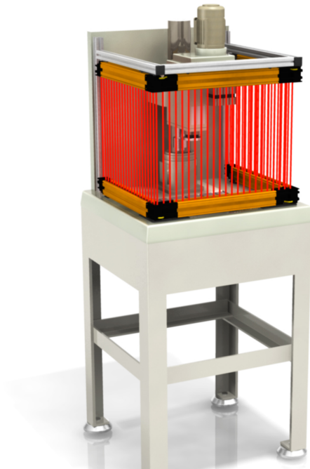
Figure 43. Cascaded light screens guarding a u-shaped cell
